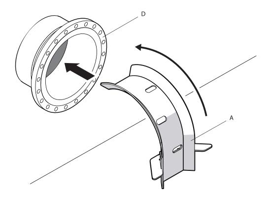
1. Make sure the curve assembly (A) is horizontally level in the manhole (D).
