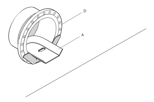
2. Use two C-clamps (F) included in the Roofac Rescue Slide package to secure the curve assembly (A) to the manhole (D).
