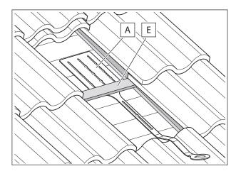
5. Use 14 metal roofing screws, 6x40 mm (F) in the 6,5 mm holes and the 8 mm holes to attach the Anchorpoint T (A) to the wood panel (G) on the roof. Use 12 screws on the upper part and 2 screws on the neck of the Anchorpoint T (A).
